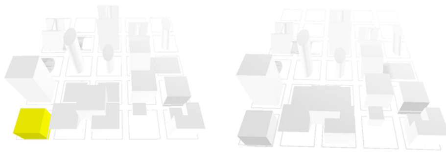
Figure 3. Case B: IFC geometries, both in IFC v.2x3 and v.4, converted to bldg:buildings , visualized in azul. It is possible to notice that, for some reason, these are inverted with respect to their original distribution.
