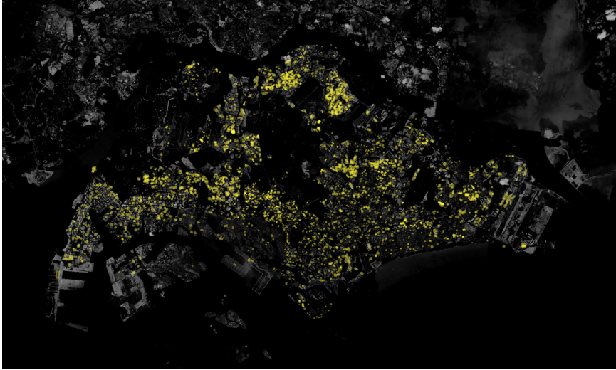
Figure 1. Locations of buildings in Singapore that have been detected to have photovoltaic installations on rooftops, using GeoAI techniques. Source: (Wu and Biljecki 2021).
