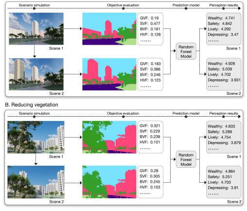
Figure 10: Demonstrations of the UDT in testing different future scenarios for predicting visual perception results.
