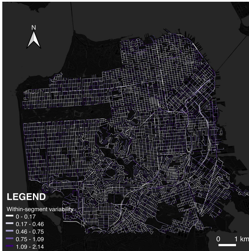
Figure A3. Spatial distribution of within-segment variability in slope across the road network. Lighter colors indicate lower variability, while darker purple denotes higher variability.
